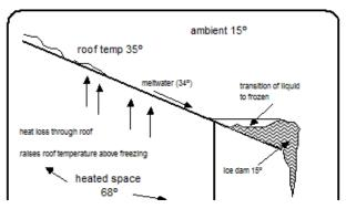
Figure 6A: The process of eave icing
