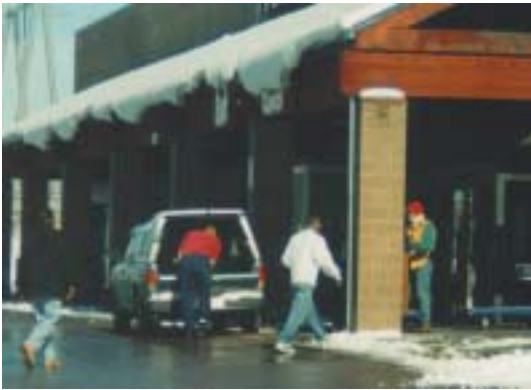
At left an unsuspecting pedestrian enters as another customer loads his truck beneath the roof eave. Moments later (right) both would have been hit by 40 or 50 pounds of snow.
