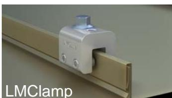
S-5!® clamps attach to the panel seam by the tightening of two "bullet-nosed" stainless steel setscrews against the seam material. (This is usually done with an industrial grade screw-gun.) The round point setscrews compress the seam material against the opposite wall of the clamp. They will "dimple" the seam material, but will not penetrate it. Threaded holes in the clamp (stainless hardware is provided) enable the easy attachment of various ancillary items to the clamps.
