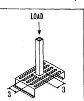
Higher loads can be supported by the transverse ribs. However, larger "foot" plates will be required to distribute the higher loads over additional ribs.
