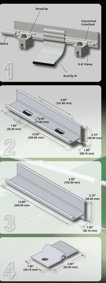
Please note: Bars come in 8' lengths, but shown here in 12" diagrams. All measurements are rounded to the second decimal place.
