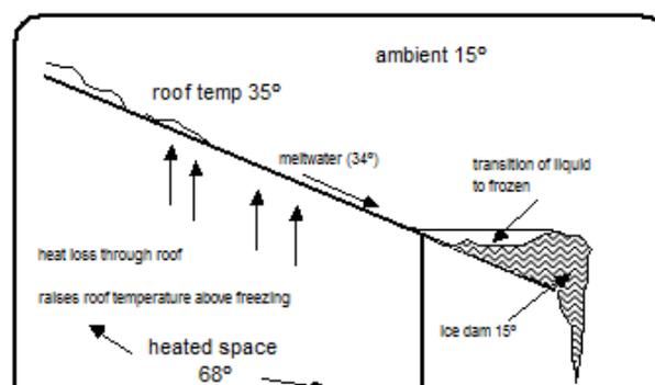
**Figure 6A: The process of eave icing**
