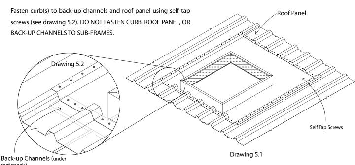
\*NOTICE\* Sub-frames and back-up channels not shown in the above picture(s).
